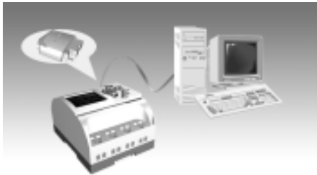
Fig.4.24. FAB Communication Connection Frame
